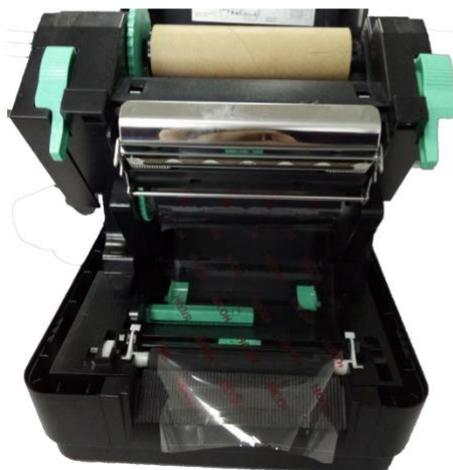
6. Insert the left side of ribbon supply spindle to the ribbon supply hub first then insert the right side of ribbon supply spindle to the hole at the right side of ribbon mechanism.
