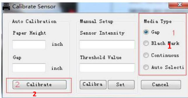
7. Use "Diagnostic Tool" to set the media sensor type and calibrate the selected sensor. (Start the "Diagnostic tool" → Select the "Printer Configuration" tab → Click the "Calibrate Sensor" button ) Please refer to section 5.3.
