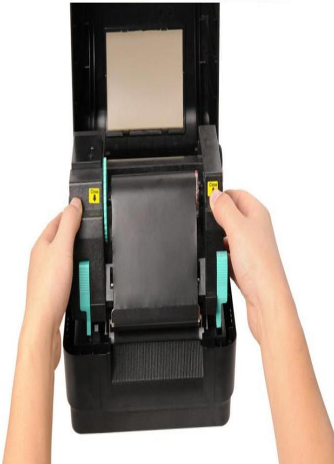
9. Close the print head mechanism by both hands and make sure the latches are engaged securely.
