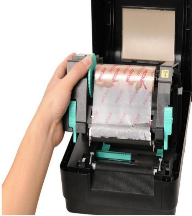
7. Pull the leader of the ribbon through the print head and stick the leader of the ribbon onto the ribbon rewind paper core.
