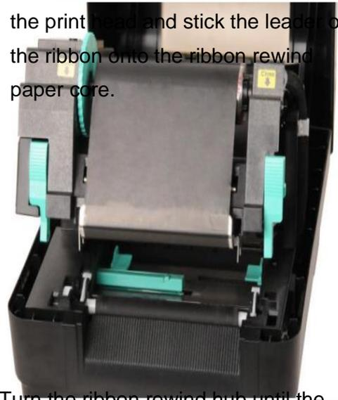
8. Turn the ribbon rewind hub until the ribbon plastic leader is thoroughly wound and the black section of the ribbon covers the print head.
