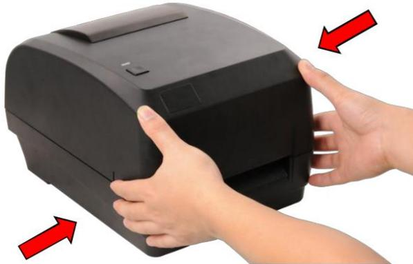
1. Open the printer top cover by pressing the top cover open tabs located on each side of the printer.
