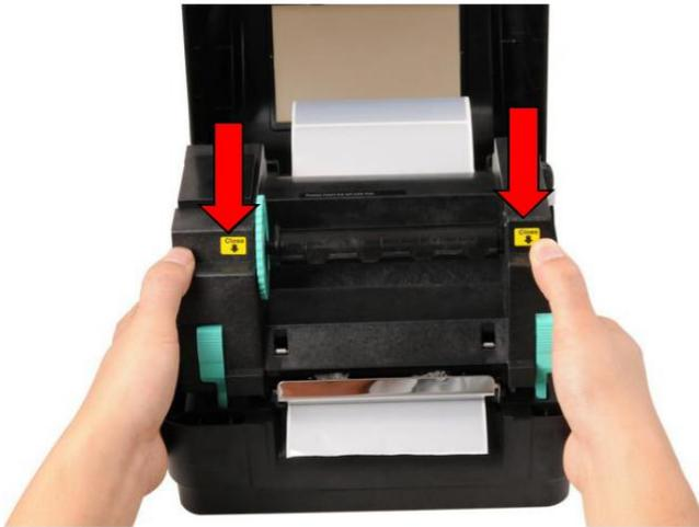
6. Close the print head mechanism by both hands and make sure the latches are engaged securely.
