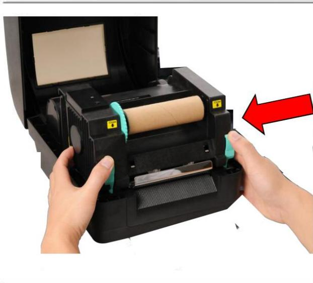
4. Push the print head release button to open the print head mechanism.
